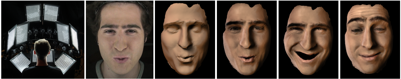
Figure 1: High resolution passive facial performance capture. From left to right: Acquisition setup; one reference frame; the reconstructed geometry (1 million polygons); final textured result; and two different frames.
